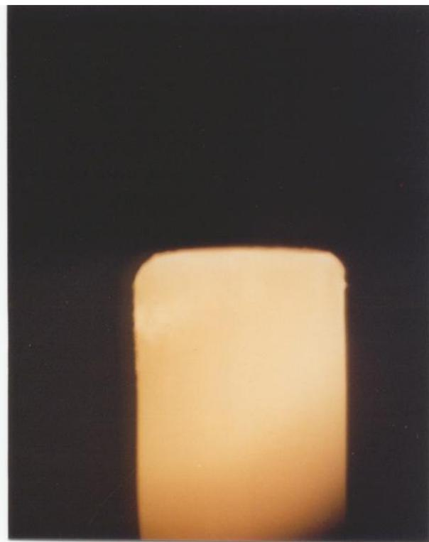
The current is distributed over the front surface of the cathode in a more or less uniform way; the **diffuse mode**.
