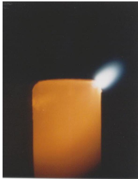
The current is localized in a region occupying a small fraction of the surface (cathode spot); a **spot mode**.
