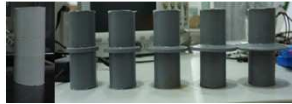
Fig. 3 Photograph of six kinds of insulators with different shed protrusion length
