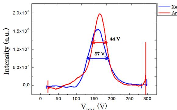
Fig.8: Comparison of Ar and Xe Ion Energy Distribution Function (IEDF)
