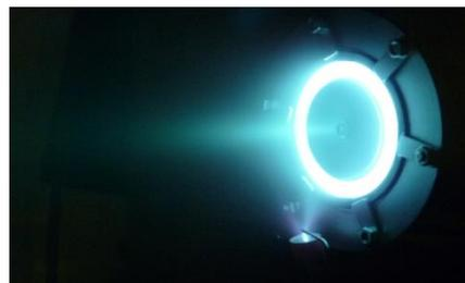
Fig.1: The PPI thruster in operation in GREMI vacuum chamber
