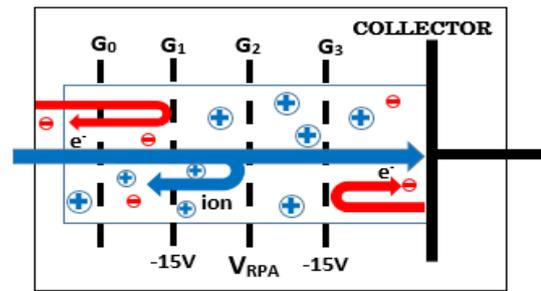
Fig.2: The schematic structure of the Retarding Potential Analyser
