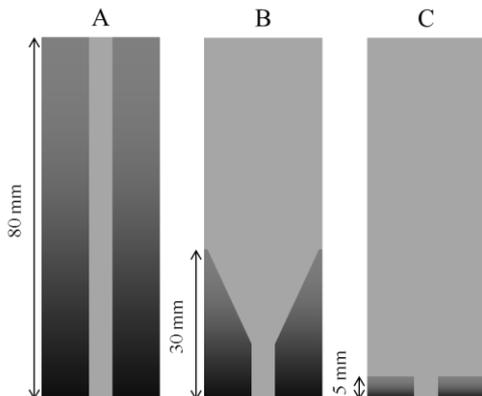
Fig. 3: Three different geometries of model spark gap [4].
