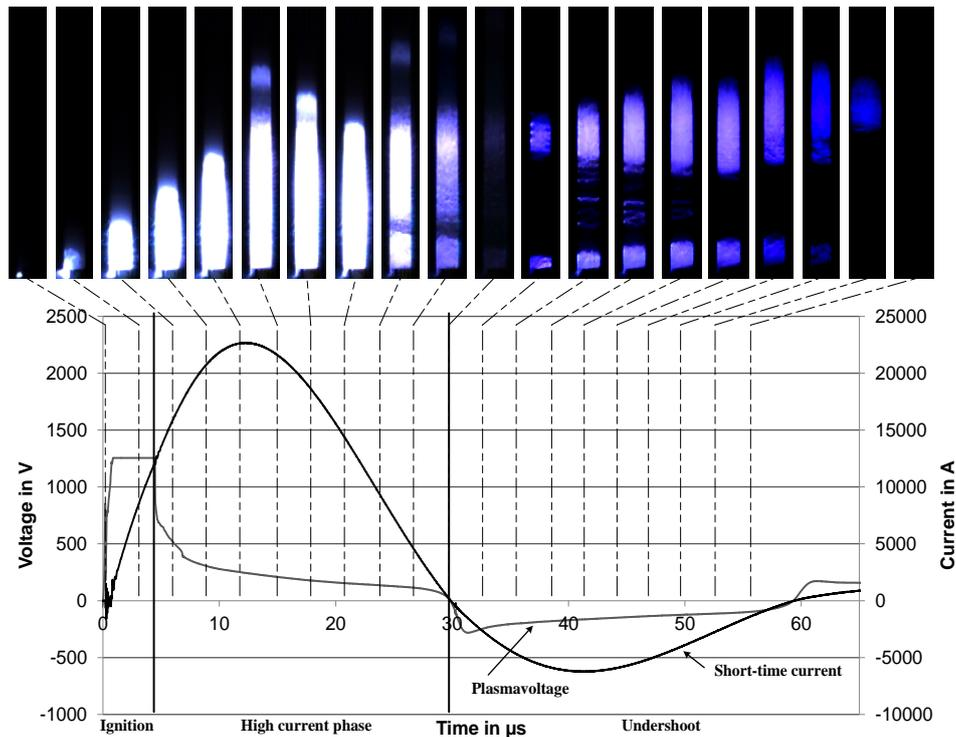
Fig. 4: Plasma propagation in a narrow gap by short-time current 23 kA, filter transparency 1,6 %, Modell spark gap A.
