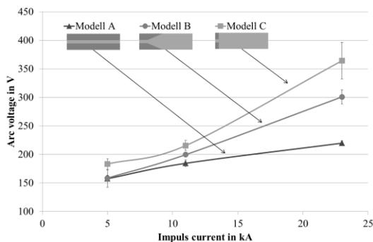
Fig. 6: Plasma voltage of three model spark gaps for different short-time currents [4].
