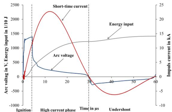
Fig. 1: Typical impulse current diagram [3].
