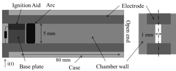
Fig. 2: Top view (left) with section line for the side view (right) of the test model [3].
