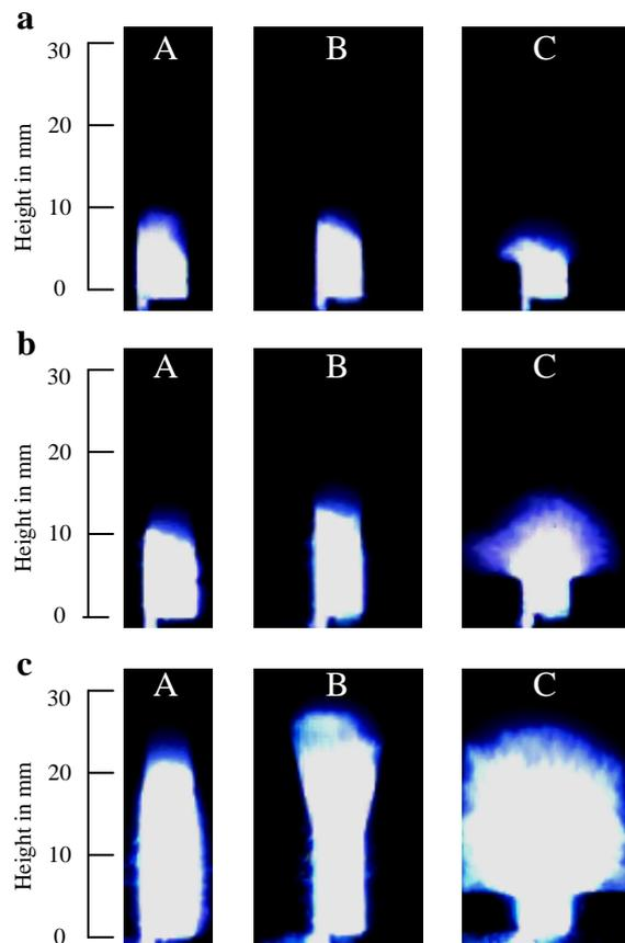
Fig.5: Plasma propagation in narrow gaps by short-time currents of 5 kA (a), 11 kA (b) and 23 kA (c) for three different geometries of electrodes, images at current maximum, filter transparency 6,25 %.
