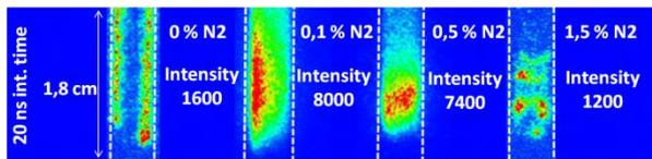
Fig. 5: ICCD images of the discharge inside the capillary (20 ns integration time) for pure helium case and 3 different % of N2. Same false color scale is used for intensity comparison (more intense in red).
