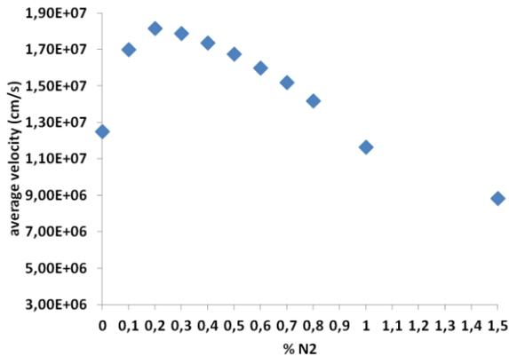
Fig. 4 : average velocity of the discharge with respect for N2 %. The average velocity is calculated here between the fiber 3 and 10.
