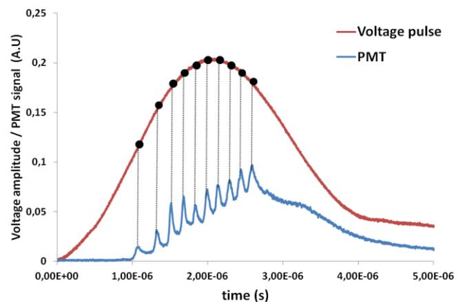
Fig. 2 : 16 kV applied voltage time profile synchronized with the PMT signal of ten optical fibers. The first fiber is located 3cm downstream from the inner electrode tip.
