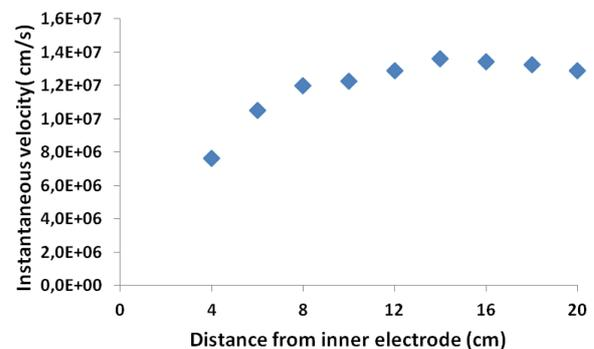
Fig 3: evolution of the velocity profile of the discharge inside the capillary. The velocity is calculated between two consecutive 2 cm spaced fibers.
