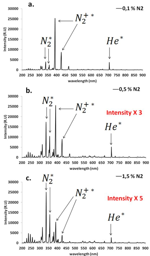
Fig. 6 : evolution of integrated (200 ms) discharge spectra through the capillary for 3 N2 % (a : 0,1%, b: 0,5%,c:1,5%)
