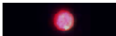
Fig. 2: Image of a discharge in a 150\ \mu\text{m} diameter cavity operated in 400 mBar of helium. The white dot at the bottom is due to the emission of an instability.
