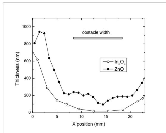
Fig. 4: Comparative thickness profile of the  $\text{In}_2\text{O}_3$  and  $\text{ZnO}$  films grown with obstacle
