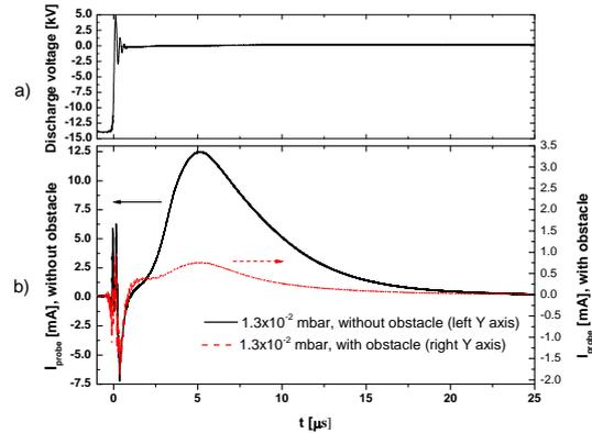
Fig. 3: a) Typical PED high voltage trace b) Ion probe signals with (straight line) and without obstacle (dotted line), at a -30V probe bias
