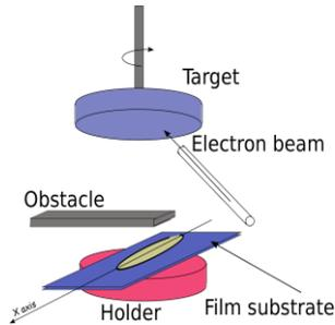
Fig. 1: Experimental setup for the film growth with obstacle
