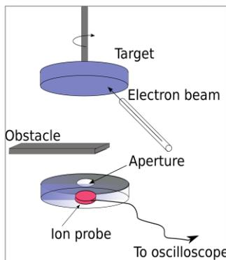
Fig. 2: Setup for ion probe measurements with obstacle
