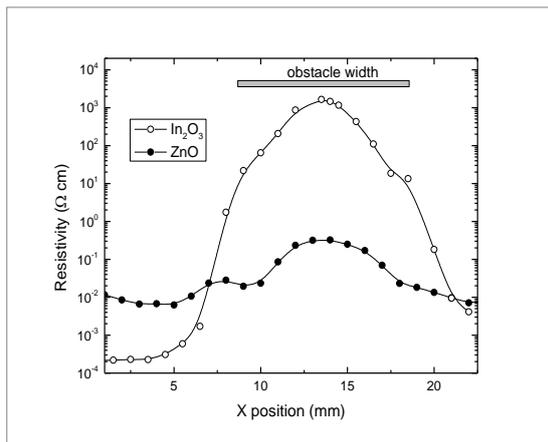
Fig 5: Comparative resistivity profile of the  $\text{In}_2\text{O}_3$  and ZnO films grown with obstacle
