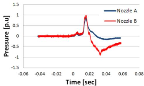
Figure 3. Measured pressure results according to different nozzle throat lengths.
