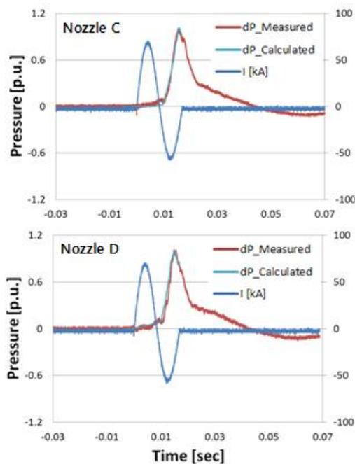
**Figure 5.** Comparison of measured and calculated results according to different nozzle shape
