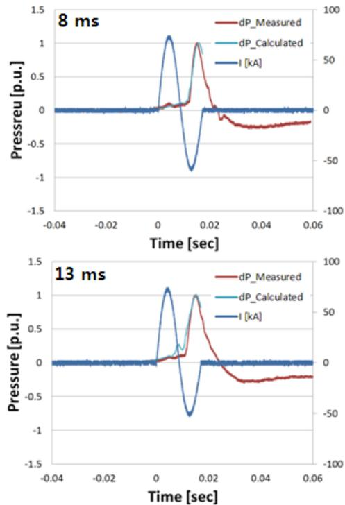
Figure 2. Comparison of the measured and experimental results by different arcing time
