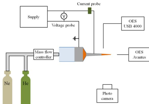
Figure 1: Experimental setup of DBD plasma jet.
