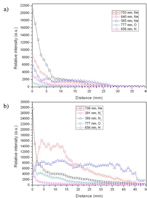
Figure 6: spatial distribution of excited species along the plasma jet for Neon a) at 1400V and 1.6 L.min<sup>-1</sup> and for Helium b) at 2400V and 3.2 L.min<sup>-1</sup>.
