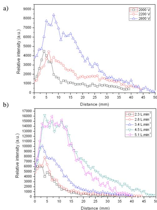
Figure 7: spatial distribution of  $N_2^+$  as a function of a) the applied voltage (at fixed flow rate) and b) the flow rate (at fixed applied voltage)
