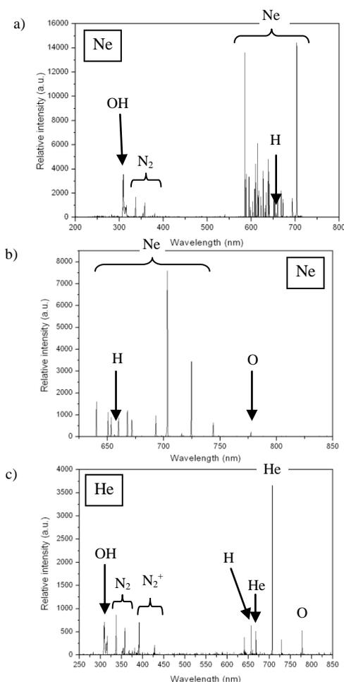
Figure 5: front spectrum: a) Neon at 1.2 L.min<sup>-1</sup>, 1700V, acquired with 500 ms integration time in a range from 250 nm to 714 nm, b) Neon at 1.2 L.min<sup>-1</sup>, 1700V, acquired with 15 ms integration time in a range from 639 nm to 850 nm, c) Helium at 3.2 L.min<sup>-1</sup>, 2300V, 200 ms integration time in a range from 250 nm to 850 nm.
