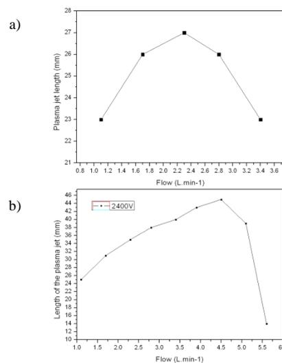
Figure 4: length of the plasma plume as function of the flow rate for Neon a) and for Helium b).
