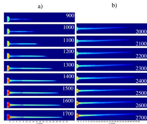
Figure 2: plasma jets for Neon a) and Helium b) as a function of the applied voltage at their own optimal flow, respectively 2.3 L.min<sup>-1</sup> and 4.5 L.min<sup>-1</sup>
