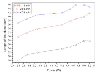
Figure 3: Length of the He plasma jet in air as function of the injected power for different flow rate
