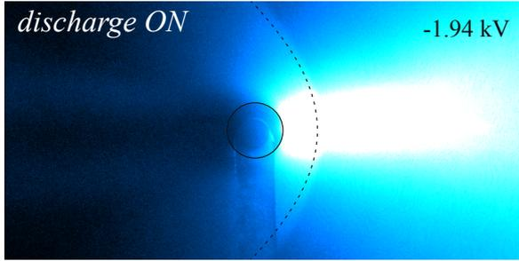
Fig. 4: ICCD image of the flow modified by the plasma discharge ( $V_{HV} = -1.94$  kV,  $I_{HV} = 100$  mA). The black line represents the shock wave shape of the natural flow (Mach 2)
