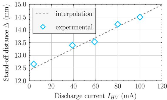
Fig. 5: Experimental stand-off  $\Delta$  estimated with the ICCD images according to the discharge current  $I_{HV}$
