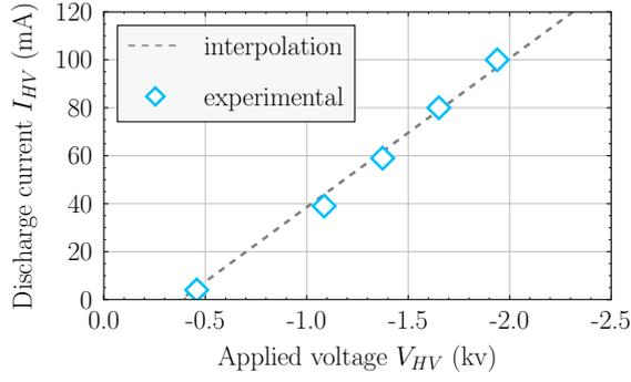
Fig. 3: Current-voltage characteristic of the discharge (Mach 2)
