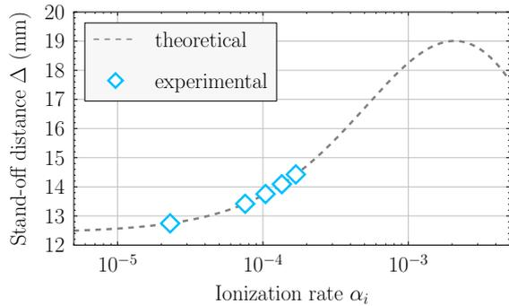
Fig. 7: Stand-off distance for a plasma according to the ionization degree. The line is the theoretical variation and the diamonds are the empirical values for the applied voltages tested experimentally
