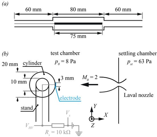
Fig. 1: Schematic representation of the cylinder in the test section: (a) front and (b) side views
