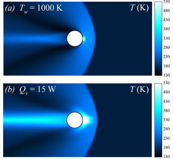
Fig. 6: Temperature fields obtained from the WENO simulations in the case of: (a) a surface heating with  $T_{w1} = 1000$  K and (b) a volumetric heating of  $Q_v = 15$  W. The Mach number is 2
