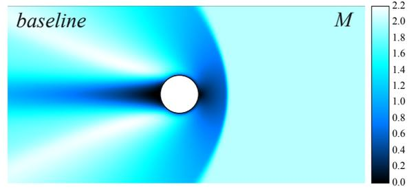
Fig. 2: Mach number field from the WENO simulation of the natural flow. The free stream Mach number is 2
