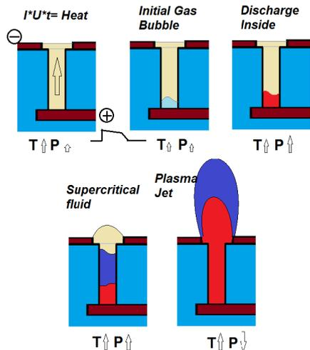
Fig. 2. Dynamic chart of supercritical injection. Yellow-initial fluid, blue-vapor bubble, red-plasma, violet-supercritical fluid and two-phase fluid.
