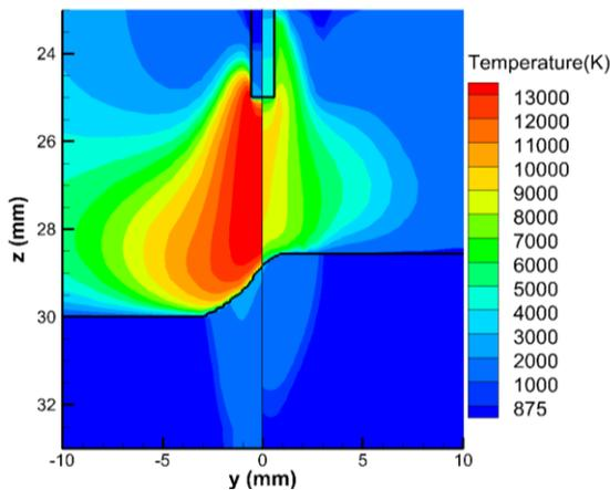
Fig. 1 Distribution of temperature in the  $x = 0$  plane including (right) and neglecting (left) the influence aluminium metal vapour. Results are for arc current 95 A, wire radius 0.6 mm, welding speed  $15 \text{ mm s}^{-1}$  in the  $-y$  direction, wire feed rate  $72 \text{ mm s}^{-1}$ , droplet detachment frequency 93 Hz, bead-on-plate welding with 3 mm thick workpiece, wire and workpiece alloy AA5745. From [3].
