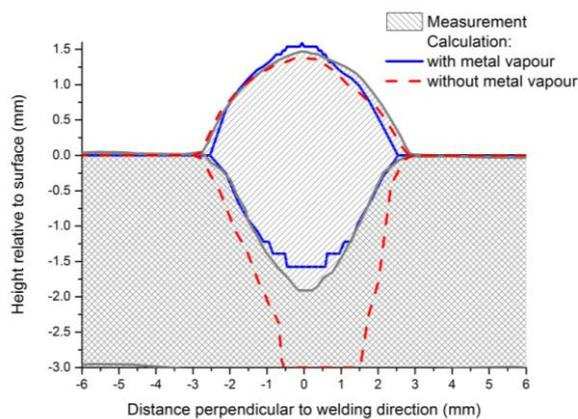
Fig. 4 Comparison of measured and predicted weld cross-sections for AA4043 wire and AA5754 workpiece alloys; other conditions are as for Fig. 1. Predictions including and excluding the influence of metal vapour are shown.
