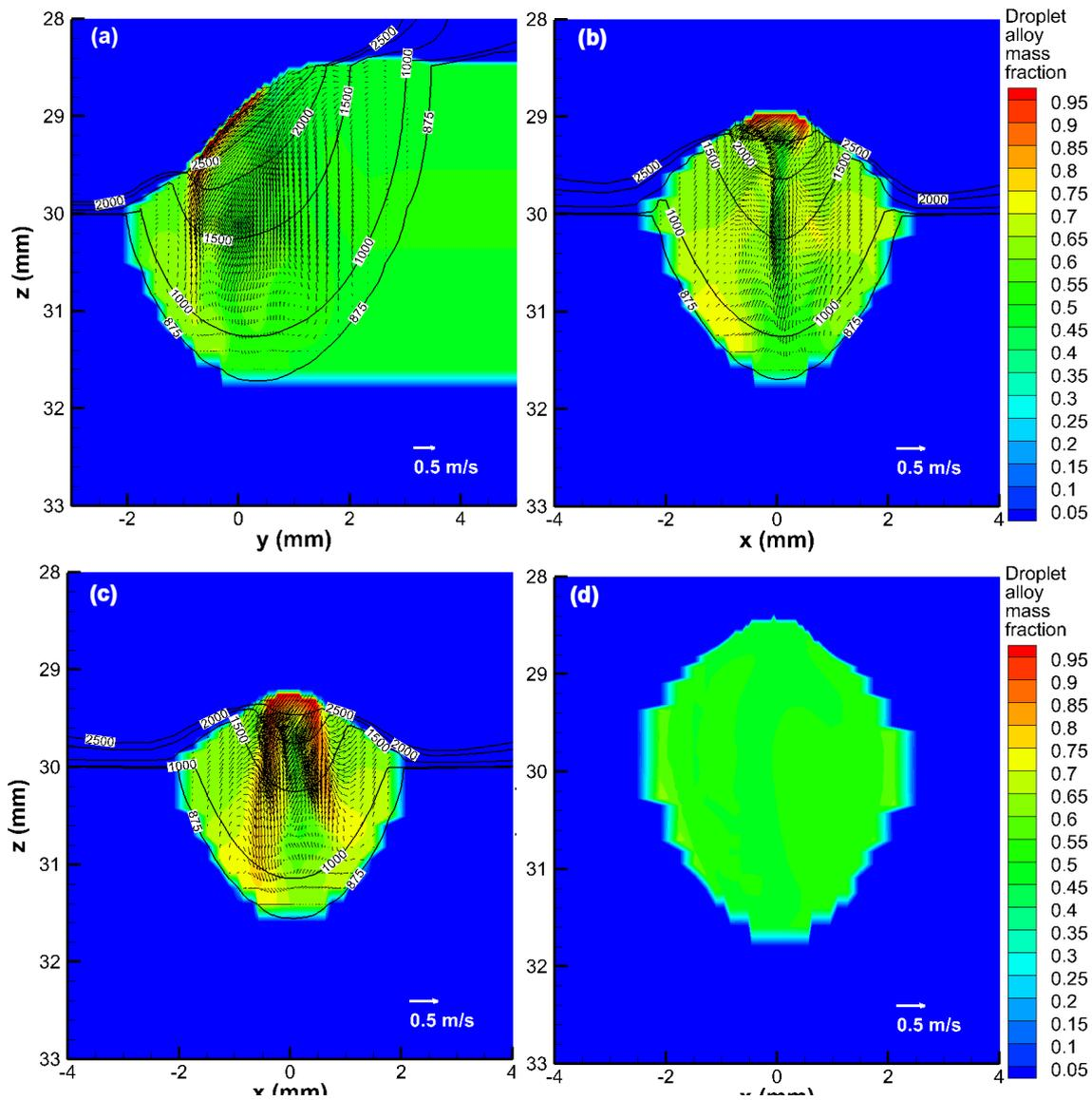
Fig. 3 Fraction of the droplet alloy in a cross-section of the weld pool, for the a)  $x = 0$  plane, b)  $y = 0$  plane, c)  $y = -0.5$  mm plane, d)  $y = 6$  mm plane. The wire is AA4043 and the workpiece alloy is AA5754; other conditions are as for Fig. 1. Velocity vectors and temperature contours for 875, 1000, 1500, 2000 and 2500 K are also shown.
