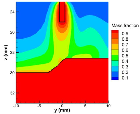
Fig. 2 Distribution of aluminium vapour mass fraction in the  $x = 0$  plane for the same conditions of Fig. 1. From [3].
