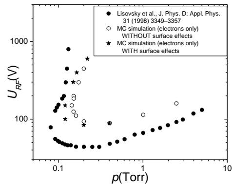
Fig. 3 Paschen curves obtained by MC code with and without surface effects included and comparison with experimental results [10]. Gap is 23mm and frequency 13.56MHz.
