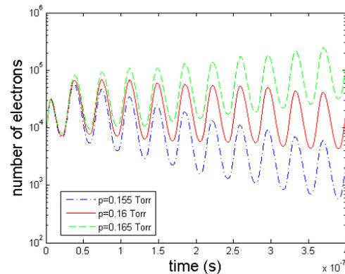
Fig. 1 Breakdown point determination. Conditions are  $U=400V$ , and pressures are:  $p_1=0.155Torr$ ,  $p_2=0.16Torr$  and  $p_3=0.165Torr$ . Background gas is argon gap 23mm and frequency 13.56MHz.
