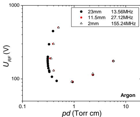
Fig. 2 Scaling law. Paschen curves for different gaps and frequencies supporting condition  $fd$ -constant.
