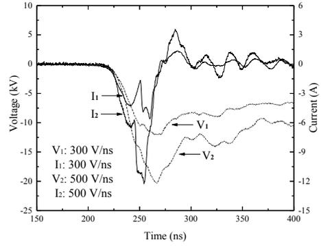
Fig. 7. The applied voltage and current through the DBD reactor when discharge even occurs
