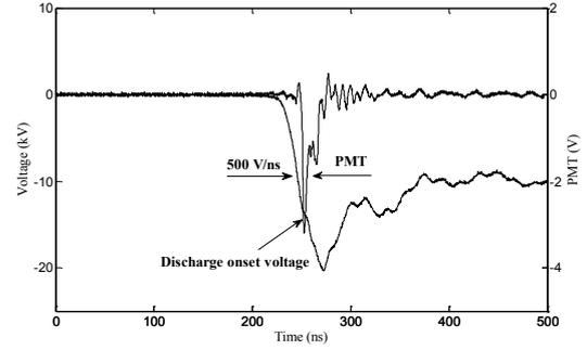
Fig. 3. Voltage impulses with 300 V/ns and 500 V/ns rise rates, and emitted light signal measured by PMT
