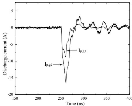
Fig. 8. The discharge current inside the discharge gap under the voltage rise rates of 300 V/ns and 500 V/ns respectively.
