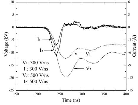
Fig. 6. The applied voltage and current through the DBD reactor when there is no discharge even
