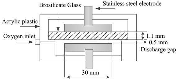
Fig 1. Schematic diagram of DBD reactor
