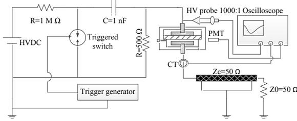
Fig. 2. Schematic diagram of electrical circuit
