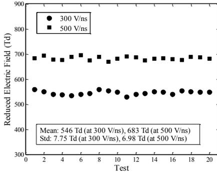
Fig. 5. The calculated reduced electric field under both voltage impulses with different rise rate
