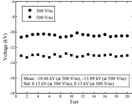
Fig. 4. The applied voltage when the discharges occur under both voltage impulses with different rise rate
