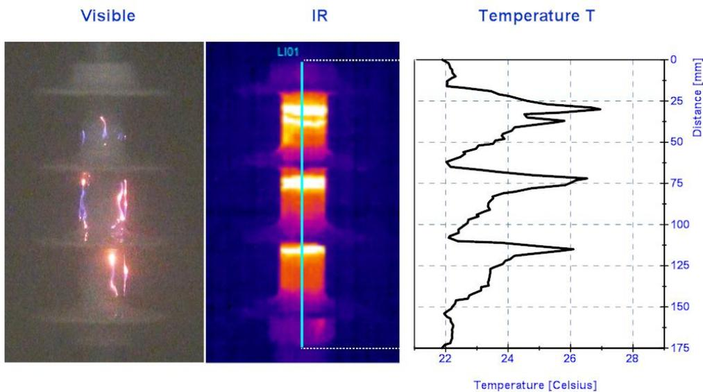
Figure 3. Visible image, infrared record and temperature profile on insulator at  $30\text{ kV}$ .
