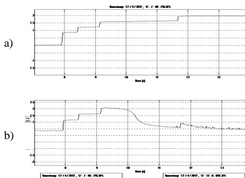
Figure 5. Dry band inception on insulator (a) Stepped applied voltage (b) Leakage current.
