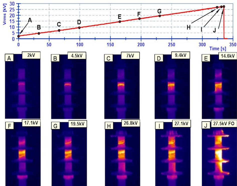
Figure 2. Formation and development of dry-bands during a ramp voltage test ( $11.2\text{ S/m}$  and  $3\text{ l/h}$ ) pollution ( $11.2\text{ S/m}$ ) and low fog ( $3\text{ litres/hour}$ ). The number and width of the dry-bands increase with the test voltage.
