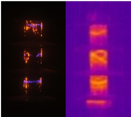
Figure 4(b). Dry-band streamers, incipient partial arcs and IR record.
