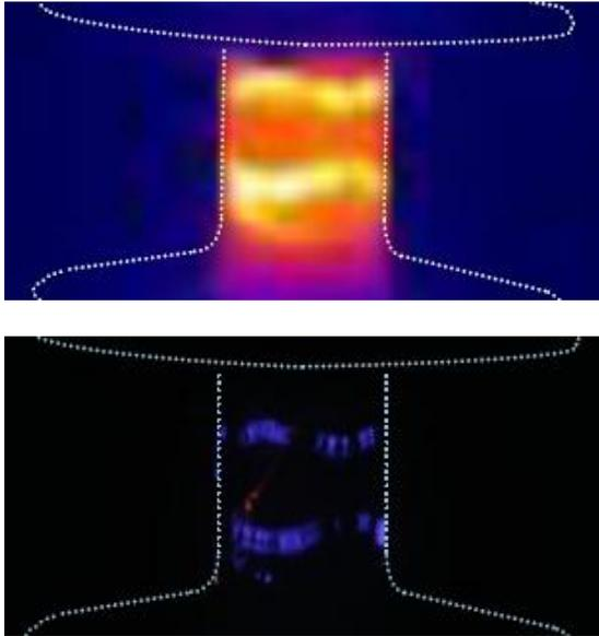
Figure 4(a). IR and visible close-ups of dry-band heating and corona discharges on the top trunk section.
