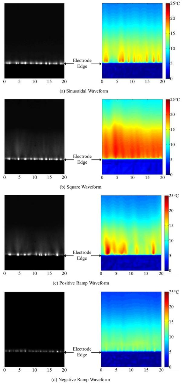
Fig. 2 Figure showing the discharge image (left) and temperature ( $\Delta T$ ) distribution (right) for (a) sinusoidal, (b) square, (c) positive ramp and (d) negative ramp waveforms. The temperatures are at  $t = 240$  s.
