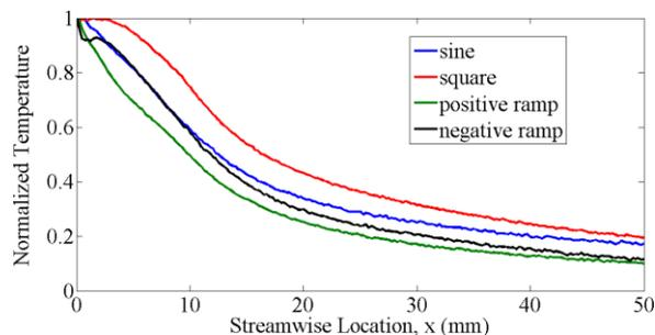
Fig. 4 Variation of temperature (normalized) downstream of the electrode for the four input waveforms. The temperatures are at  $t = 240$  s.
