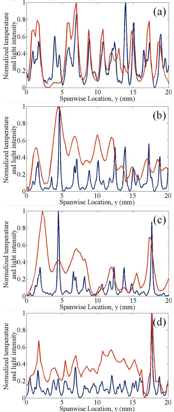
**Fig. 3** Plots of normalized temperature (red  $\rightarrow$ ) and light intensity (blue  $\rightarrow$ ) for a 20 mm span along the edge of the active electrode for (a) sine, (b) square, (c) positive ramp and (d) negative ramp waveforms. The temperatures are at  $t = 240$  s.
