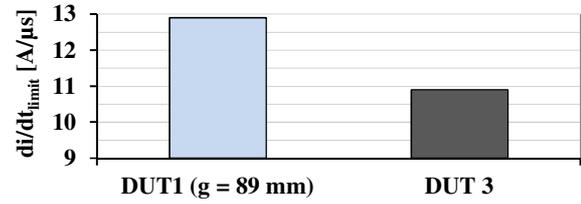
Fig. 5 Thermal interruption capability  $di/dt_{limit}$  for DUT 1 and DUT 3 at a filling pressure of  $p_{abs} = 1.0$  MPa.
