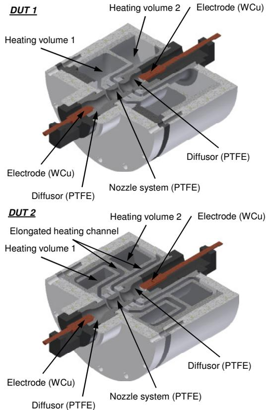
Fig. 1 Cross-sectional views of DUT 1 with two heating channels (top) and DUT 2 with elongated heating channels for increased PTFE percentage in the quenching gas (bottom).
