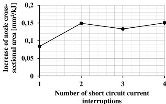
Fig. 6 Increase of the nozzle cross-sectional area in dependency of the number of short circuit interruptions
