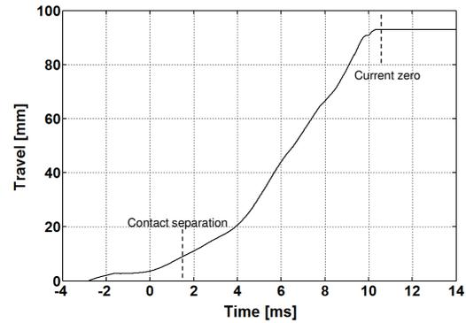
Fig. 2 Travel curve of the plug electrode in DUT 3 driven by a pneumatic operating mechanism.
