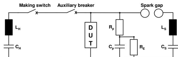
Fig. 3 Synthetic test circuit for the determination of the thermal interruption capability
