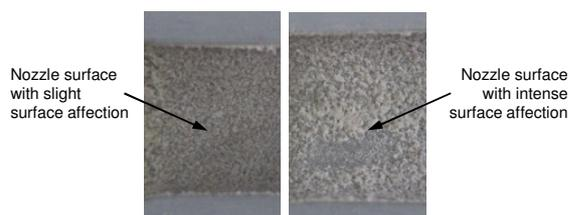
Fig. 7 Recordings of the nozzle surface after one (left) and after multiple current interruptions (right)
