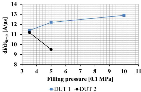
Fig. 4 Thermal interruption capability  $di/dt_{limit}$  for DUT 1 and DUT 2 for varying filling pressures (cf. [3])
