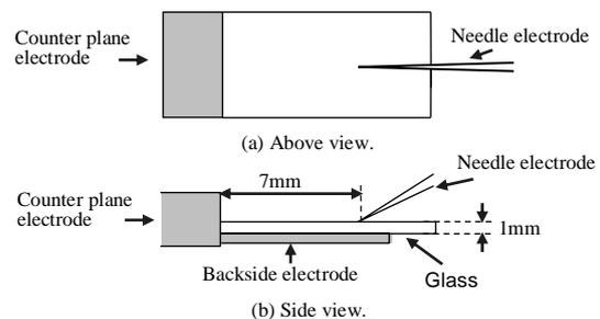
Fig. 1 Electrode configuration.
