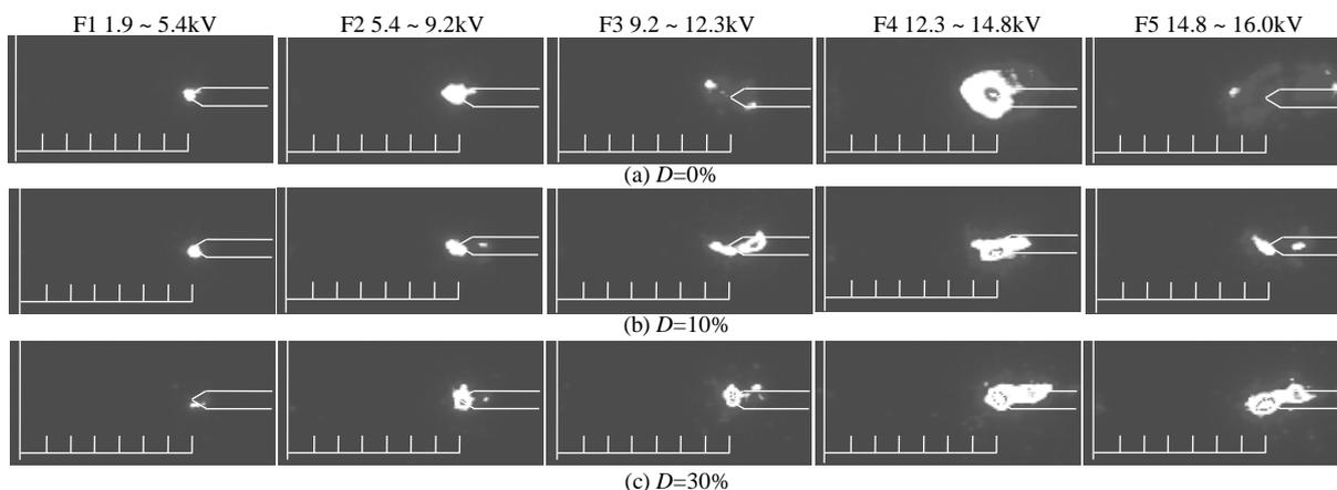
Fig.6 Creeping corona growth in  $CO_2/N_2$  by high speed camera ( $T_f=100 ns$ , Negative)
