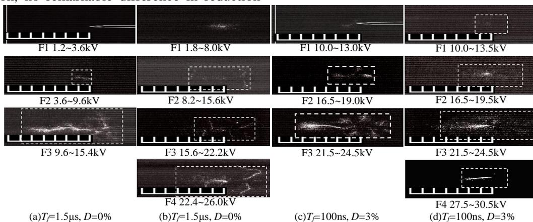
Fig.4 Creeping corona extension in  $\text{SF}_6/\text{N}_2$  by high speed camera (Negative)
