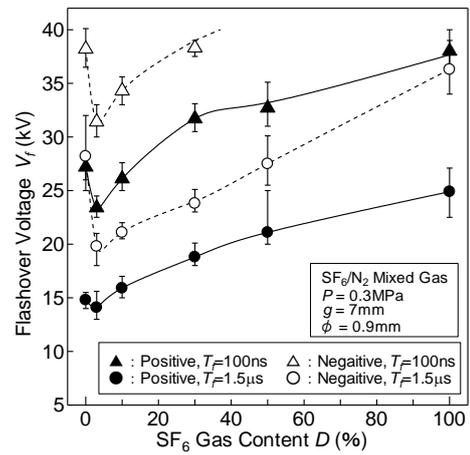
Fig.3  $\text{SF}_6$  gas content dependence of flashover voltage.
