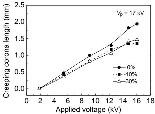
Fig.7 Applied voltage dependence of creeping corona growth
