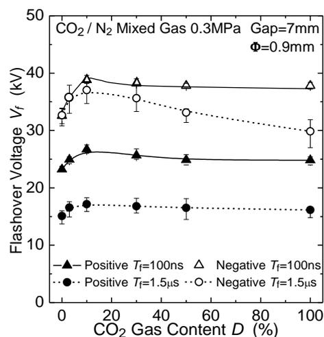
Fig. 5  $CO_2$  gas content dependence of flashover voltage.
