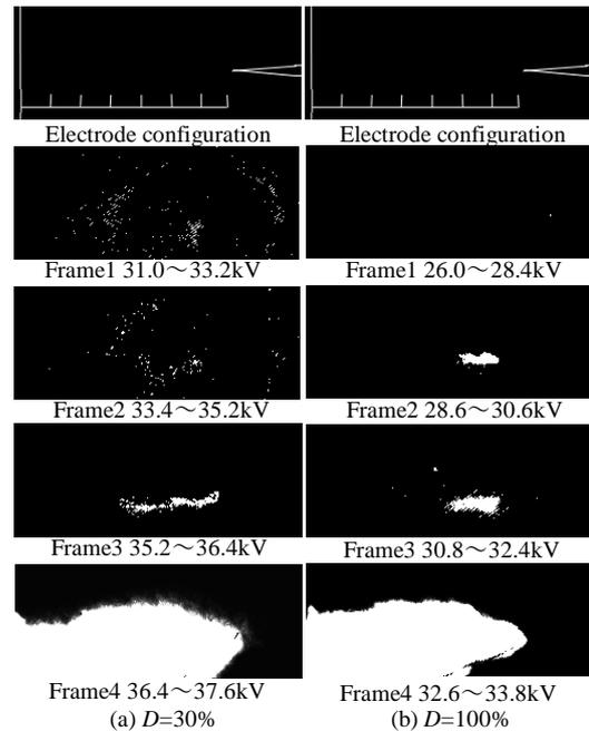
Fig.8 Creeping corona extension in  $\text{CO}_2/\text{N}_2$  ( $T_f = 1.5\mu\text{s}$ , Negative)
