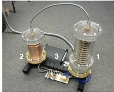
Fig. 3 High-frequency high-voltage generator, 1-inductive coupler, 2-low capacitive divider, 3-resonance converter
