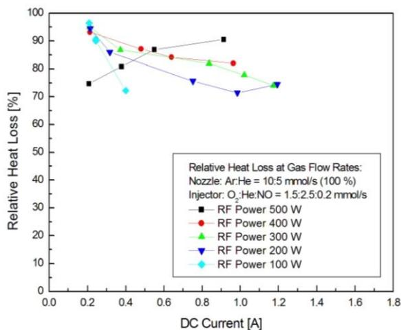
Fig. 2 Relative heat loss at standard flow rates
