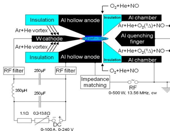
Fig. 1 Experimental scheme of DSOG-6
