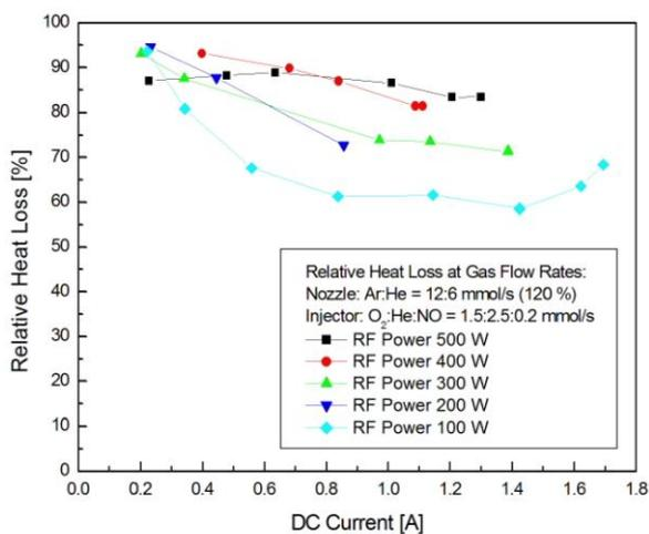
Fig. 3 Relative heat loss at increased flow rates
