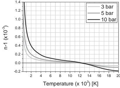
Fig. 4 Refractivity ( $n-1$ ) of air as a function of temperature for distinct values of pressure
