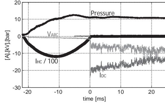
Fig. 5 Oscillograms of buffer volume pressure, high current, DC current and arc voltage recorded for a typical test shot
