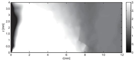
Fig. 7 Reconstructed 2D density field  $\rho(r,z)$  in  $\text{kg/m}^3$  of the observation region at the nozzle exit during the 'CZ-like' phase
