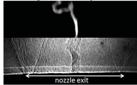
Fig. 6 Light intensity snapshot (top) and shadowgram (bottom) and obtained during the ‘CZ-like’ phase
