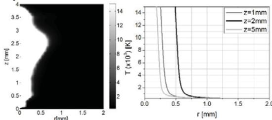
Fig. 8 (Left) Reconstructed 2D temperature field  $T(r,z)$  in  $(\times 10^3)\text{K}$  and radial plots of temperature for distinct  $z$ -positions
