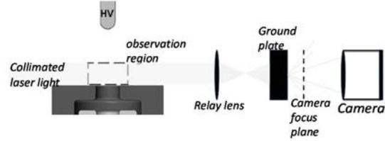
Fig. 3 Schematic of the optical setup for Speckle diagnostics
