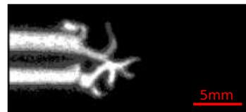
Fig. 2: Fast imaging of the plasma jet at the tube outlet with an ICCD camera. Time of exposure:  $1\mu\text{s}$
