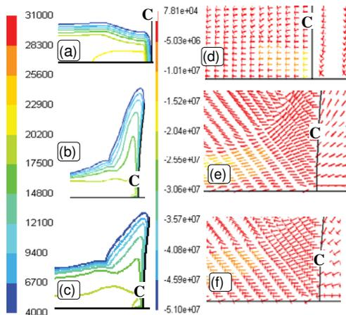
Fig. 4: (a-c) Temperature contour and Current density vectors (colored by radial Lorentz forces)-near the Cathode for (a,d) flat, (b,e) hemi-spherical and (c,f) elliptical tip of the electrodes
