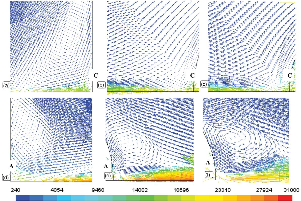
Fig. 3: Velocity vectors - colored by temperature - near the (a-c) Cathode and (d-f) Anode for (a,d) flat, (b,e) hemi-spherical and (c,f) elliptical tip of the electrodes
