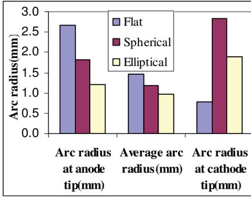
Fig. 6: Comparison of arc-radius for the various shapes of the tip of the electrodes.
