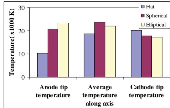
Fig. 5: Comparison of temperature for the various shapes of the tip of the electrodes
