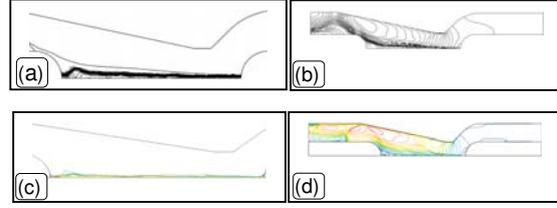
Fig. 2: Validation of numerical methodology for small current interruption, with 300A arc struck between semi-hemispherical tip electrodes: Contours of (a,c) temperature and (b,d) Mach number, with the range of variation for the respective variable as 228K-27130K and 0.00488-2.395 in the (a,b) published[1] and as 247.85K- 28217.4K and 0.0049-2.47 in the (c,d) present results.
