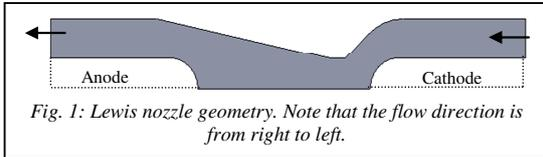
Fig. 1: Lewis nozzle geometry. Note that the flow direction is from right to left.
