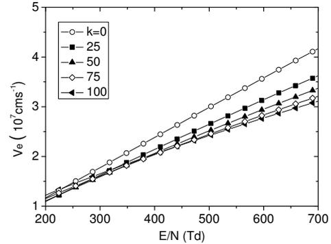
Fig. 2: The electron drift velocities in  $\text{CF}_3\text{I}$  and Xe mixtures as a function of  $E/N$  at different  $\text{CF}_3\text{I}$  gas mixture ratio  $k(\%)$ .
