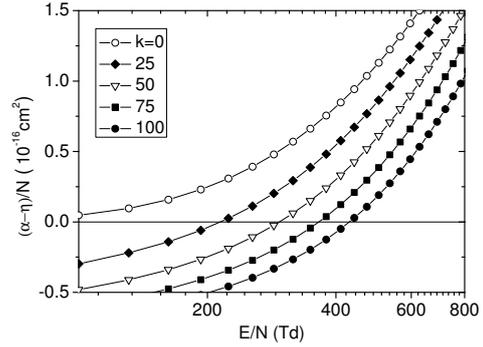
Fig. 1: The density-normalized effective ionization coefficients of  $\text{CF}_3\text{I}$  and Xe mixtures as a function of  $E/N$  at different  $\text{CF}_3\text{I}$  gas mixture ratio  $k(\%)$ .
