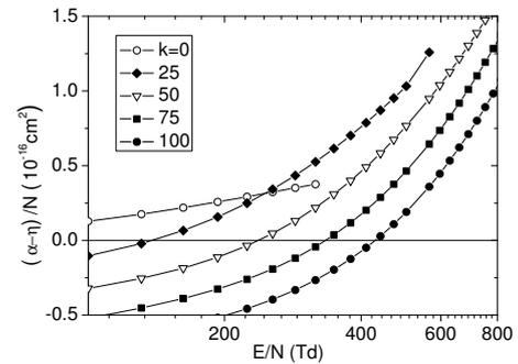
Fig. 3: The density-normalized effective ionization coefficients of  $\text{CF}_3\text{I}$  and He mixtures as a function of  $E/N$  at different  $\text{CF}_3\text{I}$  gas mixture ratio  $k(\%)$ .
