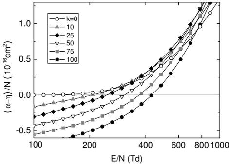
Fig. 5: The density-normalized effective ionization coefficients of  $\text{CF}_3\text{I}$  and  $\text{N}_2$  mixtures as a function of  $E/N$  at different  $\text{CF}_3\text{I}$  gas mixture ratio  $k$ (%).
