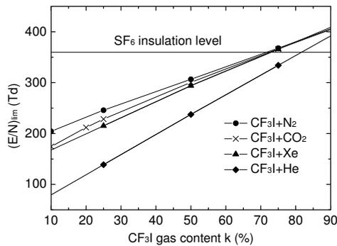
Fig. 9: The limiting fields  $(E/N)_{lim}$  as a function of  $\text{CF}_3\text{I}$  gas content  $k$ .
