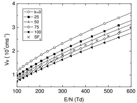
Fig. 8: The electron drift velocities in  $\text{CF}_3\text{I}$  and  $\text{CO}_2$  mixtures as a function of  $E/N$  at different  $\text{CF}_3\text{I}$  gas mixture ratio  $k$ (%).
