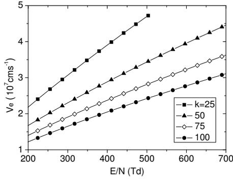
Fig. 4: The electron drift velocities in  $\text{CF}_3\text{I}$  and He mixtures as a function of  $E/N$  at different  $\text{CF}_3\text{I}$  gas mixture ratio  $k$ (%).
