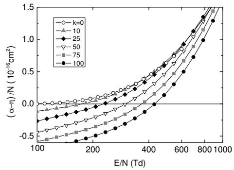
Fig. 7: The density-normalized effective ionization coefficients of  $\text{CF}_3\text{I}$  and  $\text{CO}_2$  mixtures as a function of  $E/N$  at different  $\text{CF}_3\text{I}$  gas mixture ratio  $k$ (%).
