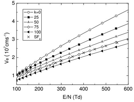
Fig. 6: The electron drift velocities in  $\text{CF}_3\text{I}$  and  $\text{N}_2$  mixtures as a function of  $E/N$  at different  $\text{CF}_3\text{I}$  gas mixture ratio  $k$ (%).
