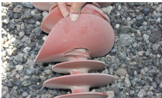
Fig. 1 shed crack of the composite insulator at 750kV Urumqi-Turpan Lines
