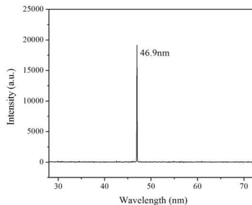
Fig. 4 Time-integrated axial emission spectrum, showing Ne-like Ar laser line at 46.9 nm.
