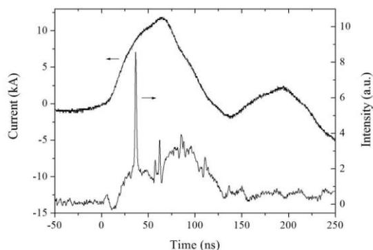
Fig. 1 Discharge current pulse and temporal evolution of soft x-ray emission detected by XRD. The Ar pressure was 12.5 Pa
