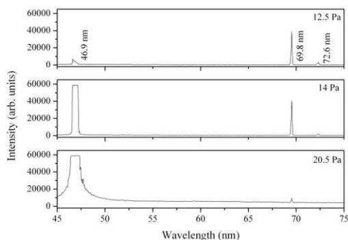
Fig. 2 Time-integrated axial emission spectra, showing three Ne-like Ar laser lines at 46.9 nm, 69.8 nm and 72.6 nm.
