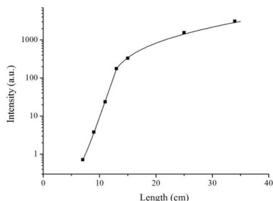
Fig. 7 Variation of the intensity of 46.9 nm line as a function of plasma column length. A fit to the Linford formula yields a gain coefficient of  $1.0 \text{ cm}^{-1}$ .
