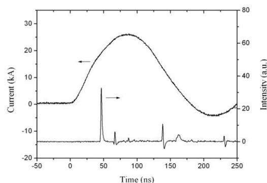
Fig. 6 Discharge current pulse and 46.9 nm laser output pulse
