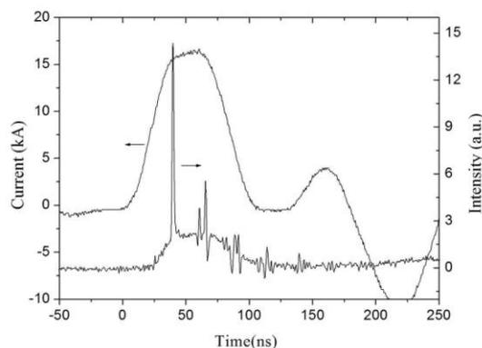
Fig. 3 Discharge current pulse and temporal evolution of soft x-ray emission detected by XRD
