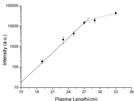
Fig. 5 Variation of the intensity of 46.9 nm line as a function of plasma column length. The gain coefficient determined by Linford formula is  $0.58 \text{ cm}^{-1}$ .
